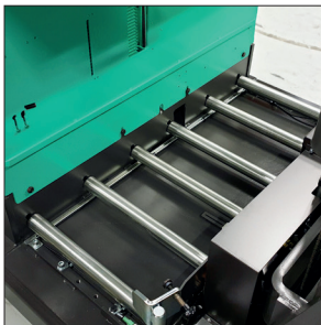
Battery on steel rollers
