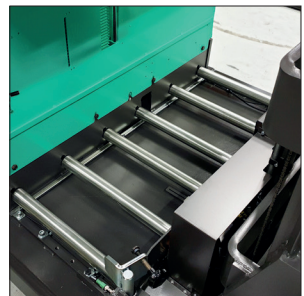
Battery on steel rollers
